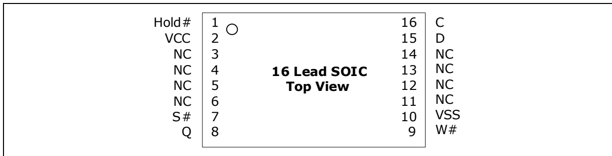
Figure 4: SOIC-16 Package Pinout
