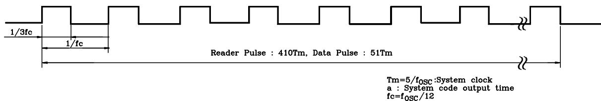
When oscillation frequency is 455kHz, signal is output after pulse modulated by 37.9kHz of duty 1/3, which is a 1/12 division by the carrier generation circuit.
