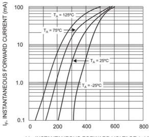
V<sub>F</sub>, INSTANTANEOUS FORWARD VOLTAGE (mV) Fig. 2 Typical Forward Characteristics
