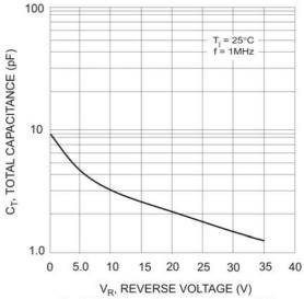
Fig. 4 Total Capacitance vs. Reverse Voltage
