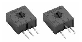
The Model 63 cermet trimmer is available in several pin configurations for top or side adjustment and with a choice of Knob styles for finger setting. Quick adjustment is achieved with multi-finger wiper and the standard resistance range is between 100  $\Omega$  and 2 M $\Omega$  with a tolerance of  $\pm$  10 %.
