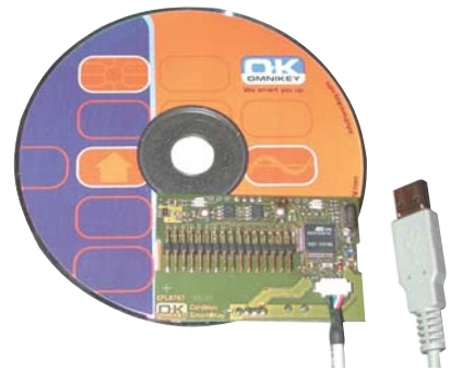
AT83C22OK/23OK Reference Design
