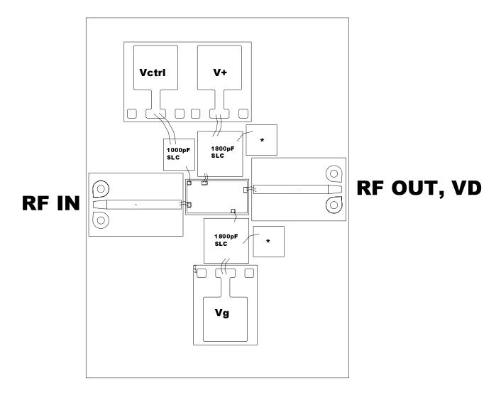
Note: Input and Output ports are DC coupled.
