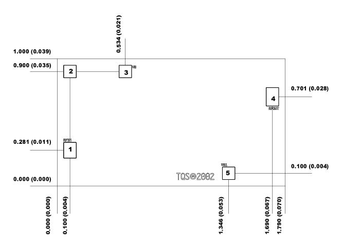
Units: millimeters (inches) Thickness: 0.100 (0.004) (reference only) Chip edge to bond pad dimensions are shown to center of pad Chip size tolerance: +/- 0.051 (0.002)
