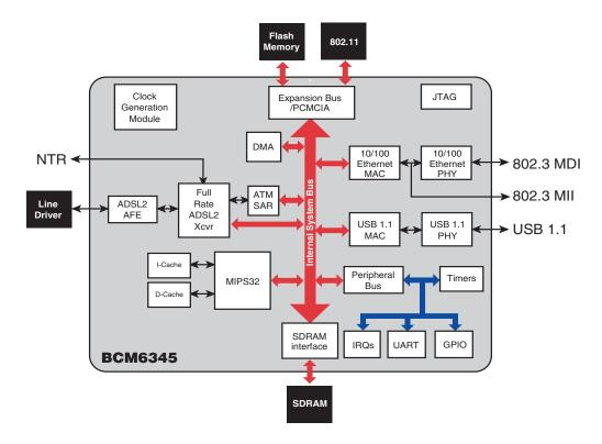
The BCM6345 combines a G.992.1/G.992.2/G.992.3/T1.413-compliant ADSL2 transceiver and AFE with a high-performance MIPS32<sup>™</sup> CPU, 10/100 Ethernet and USB 1.1 interfaces, PCMCIA and programmable 16-bit external bus interfaces into a single chip.
