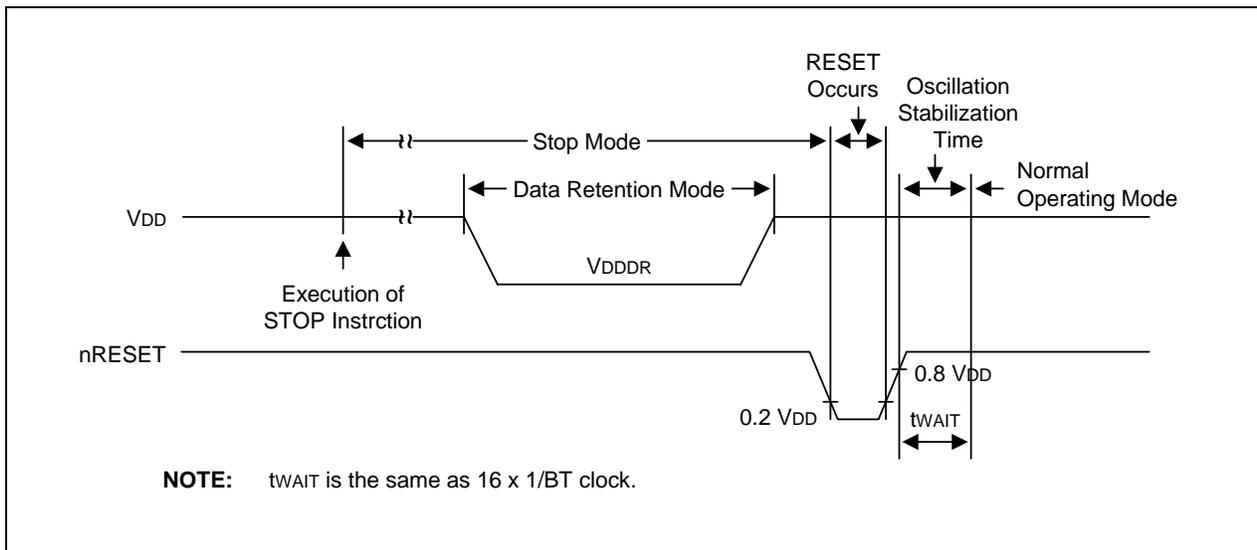
Figure 13-3. Stop Mode Release Timing Initiated by RESET
