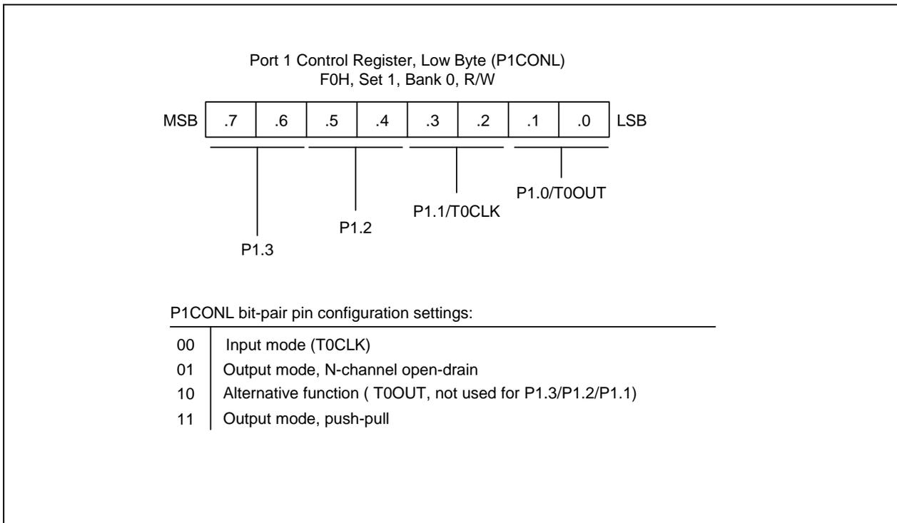
**Figure 9-6. Port 1 Low-Byte Control Register (P1CONL)**
