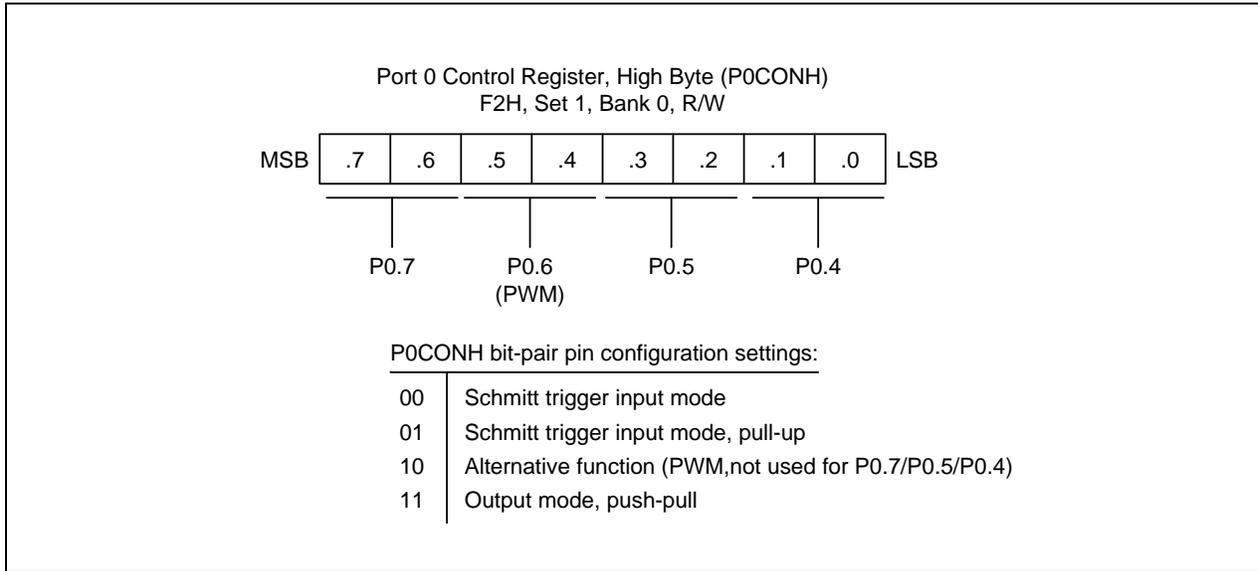
**Figure 9-1. Port 0 High-Byte Control Register (P0CONH)**
