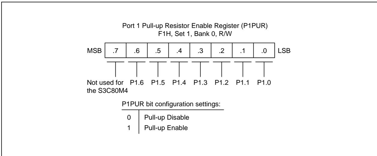
**Figure 9-7. Port 1 Pull-up Resistor Enable Register (P1PUR)**
