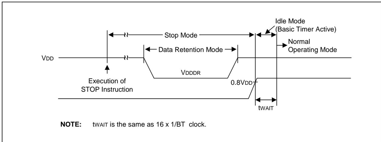
Figure 13-4. Stop Mode Release Timing Initiated by Interrupt
