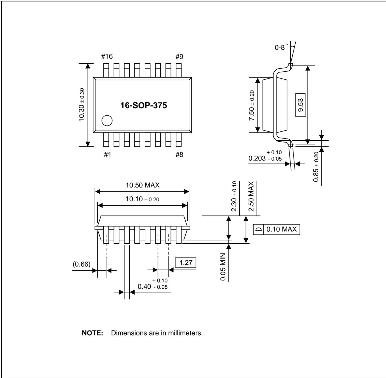
**NOTE:** Dimensions are in millimeters.
