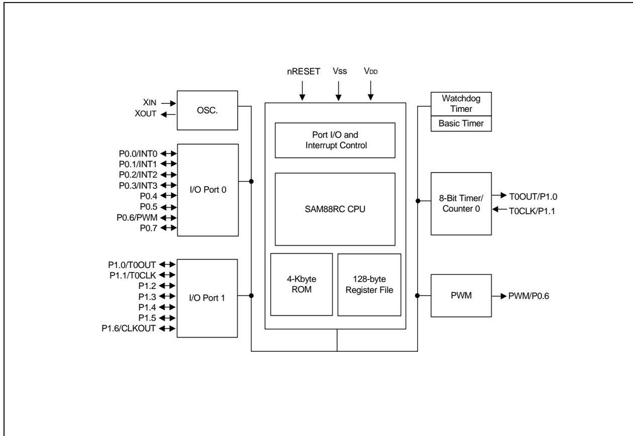
Figure 1-1. Block Diagram
