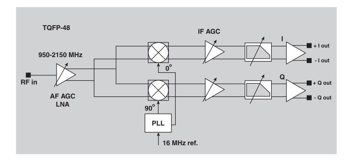
The BCM3440 is a highly integrated CMOS tuner for the direct broadcast satellite (DBS) market. It is designed to operate with Broadcom's Advanced Modulation Receiver, the BCM4500, which supports 8PSK modulation with turbo code FEC. The BCM3440 also operates with the BCM4201 QPSK satellite receiver. It is designed to support the full 1–45 Mbaud DVB operating range with support for 950 to 2150 MHz input frequencies.
