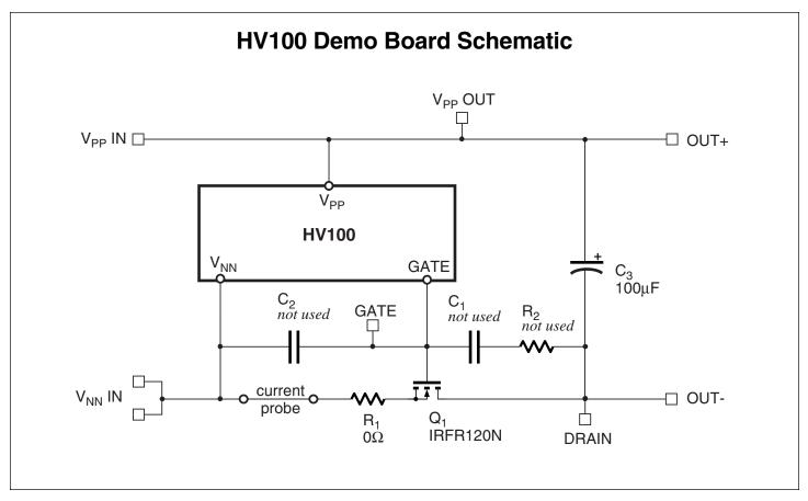
A very high dV/dt on the input can overload the HV100's internal gate clamp, causing turn-on transients. A capacitor in the  $C_2$  position may be used to clamp the gate, preventing the transients. A 1nF value is usually adequate. Voltage rating should be 16 volts.
