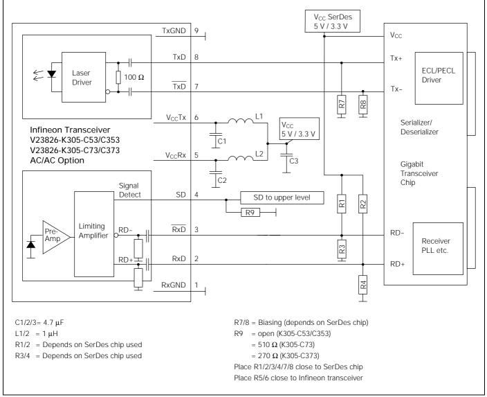
Values of R1/2/3/4 may vary as long as proper 50  $\Omega$  termination to V<sub>EE</sub> or 100  $\Omega$  differential is provided. The power supply filtering is required for good EMI performance. Use short tracks from the inductor L1/L2 to the module V<sub>CC</sub>Rx/V<sub>CC</sub>Tx.
