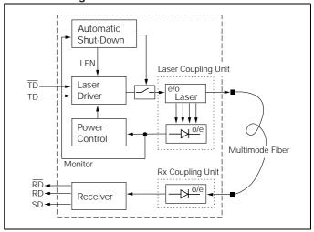
The receiver component converts the optical serial data into PECL compatible electrical data (RD and RDnot). The Signal Detect (SD, active high) shows whether an optical signal is present.
