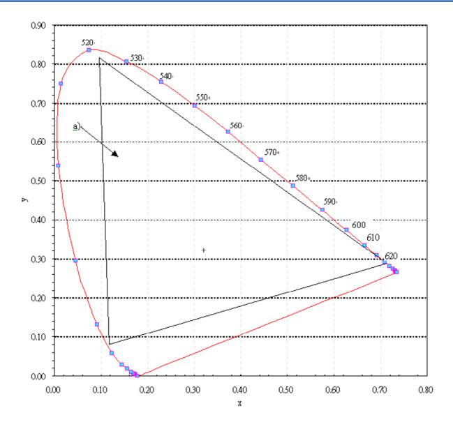
The color coordinates of the mixed light can be expected within the area of the color triangle marked "a)". The achromatic point (x=0.33,y=0.33) is marked "+".
