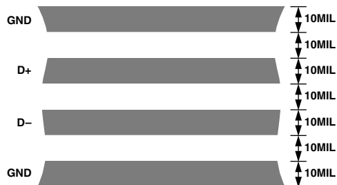
Figure 8. Arrangement of Signal Tracks
