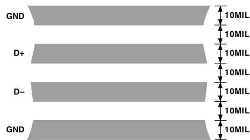
Figure 4. Arrangement of Signal Tracks
