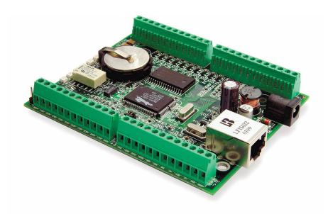
For the most demanding applications, the BL2000 and BL2020 models include 4 channels of 12-bit resolution A/D input, 5 channels of dual-purpose input, and 2 channels of 12-bit D/A output. For applications not requiring high-resolution analog I/O, the BL2010 and BL2030 offer 4 channels of 10-bit resolution A/D input and 7 channels of dual-purpose input. The dual-purpose inputs are software configurable as analog inputs or programmable-threshold digital inputs.
