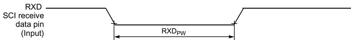
Figure 10-16 RXD Pulse Width
