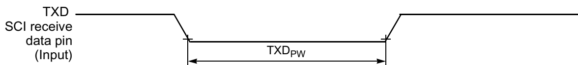
Figure 10-17 TXD Pulse Width
