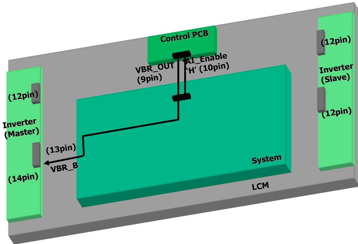
Fig. AI Application By-pass on System Board
