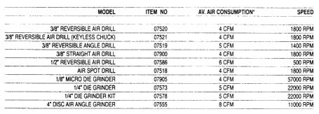
EACH TOOL COMES COMPLETE WITH ITS OWN INDIVIDUAL SUPPLY OF LUBRICANT, 1/4" BSP INLET AND REQUIRES A RECOMMENDED AIR PRESSURE OF 90 PSI (6.2 BAR) CONSUMABLES AVAILABLE - SEE PRICE LIST
