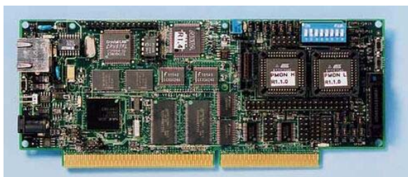
VR4131 CPU Board (75 mm × 180 mm)
