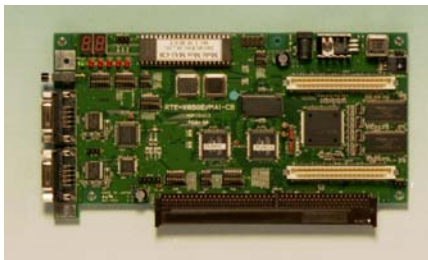
V850E/MA1 CPU Board (110 mm × 200 mm)
