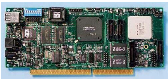
VR5500 CPU Board (84 mm × 184 mm)
