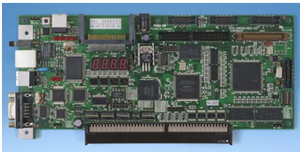
V850E/ME2 CPU Board (107 mm × 237 mm)
