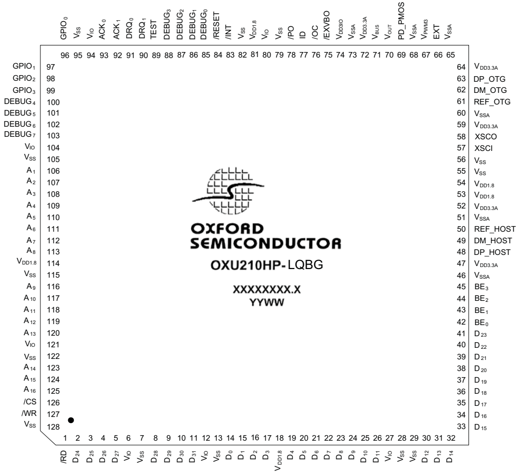
Figure 2 OXU210HP 128-Pin LQFP Package (Top View)
