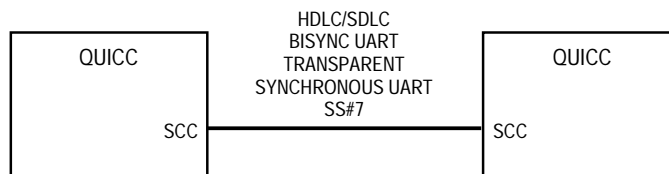
Figure 1-15. Multiple QUICC Point-to-Point Implementation
