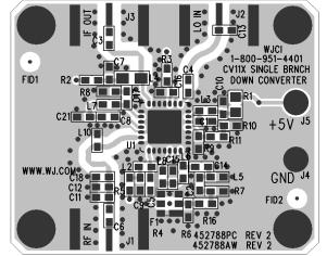
Circuit Board Material: .014" FR-4, 4 layers, .062" total thickness
