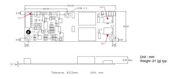
Note: Please use plastic screw in case of a non-insulating mounting base!
