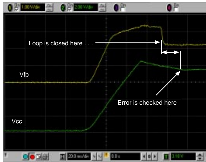
Figure 6. It is Important to Check for a Safe Start–Up Sequence
