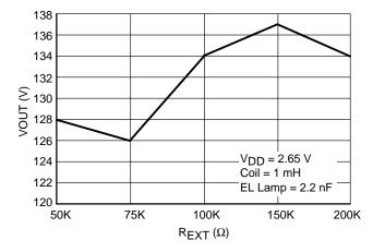
Figure 8. Output Voltage versus REXT
