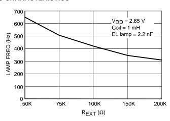
Figure 5. Lamp Frequency versus REXT
