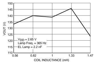
Figure 9. Output Voltage versus Coil Inductance
