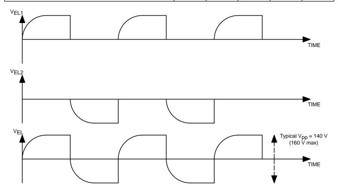
Figure 2. Output Waveform
