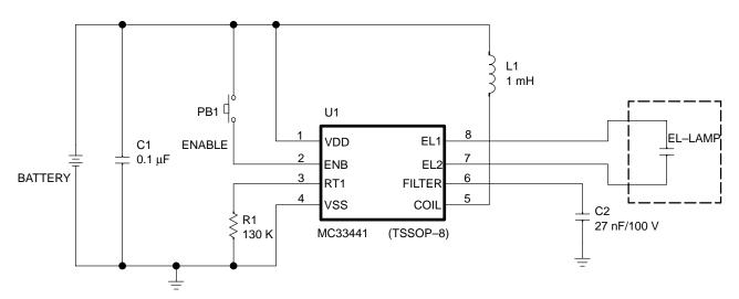
Figure 10. MC33441 Demo Board Schematic
