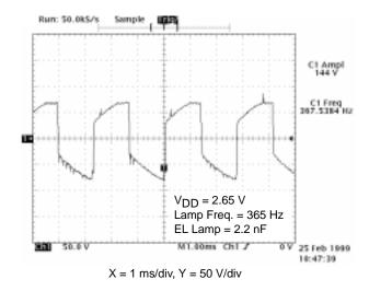
Figure 3. Output Waveform versus Time
