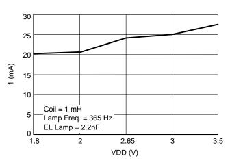
Figure 7. Current Consumption versus VDD
