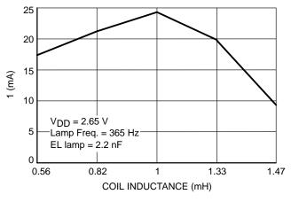
Figure 6. Current Consumption versus Coil Inductance
