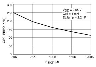
Figure 4. Oscillator Frequency versus REXT
