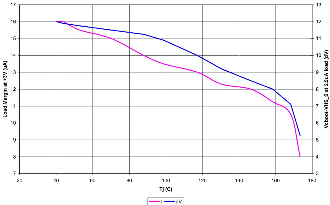
Figure 12. Typical Voltage and Load Margin For Increasing Junction Temperature at 14 V on HS\_S
