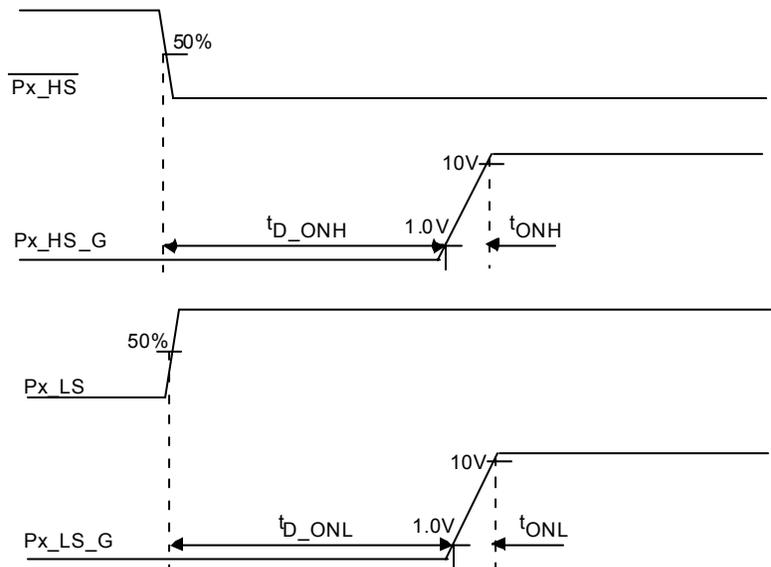
Figure 7. Driver Turn-On Time and Turn-On Delay
