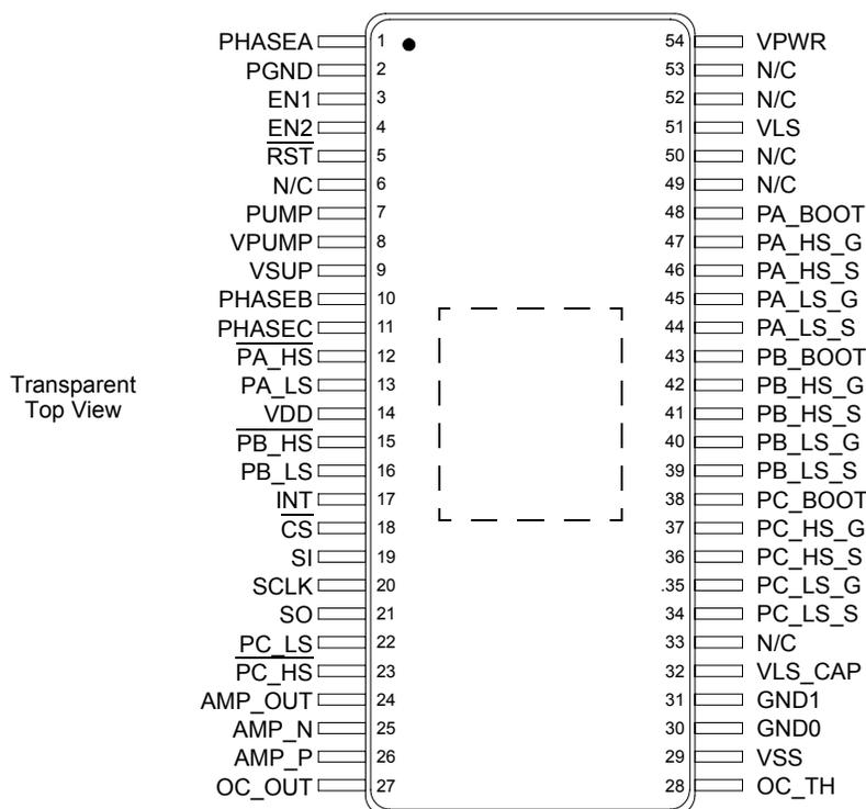
Figure 3. 33937 Pin Connections
