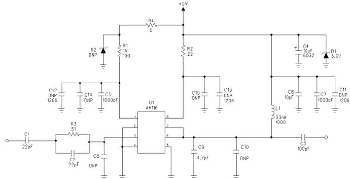
C9 is placed at the silkscreen marker '11' or center of component placed at 29 deg. @ 960 MHz away from pin 6. DNP represents "Do not populate".
