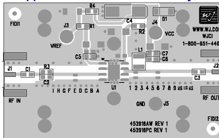
Circuit Board Material: .014" Getek, 4 - layer, 1 oz copper, Microstrip line details: width = .026", spacing = .026"
