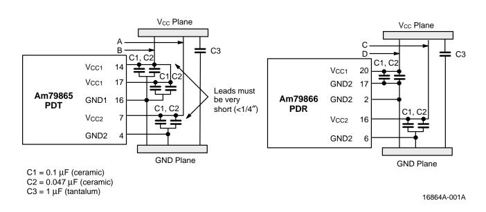
To further decouple the power supplies, ferrite beads may be used at locations A, B, C, and D.
