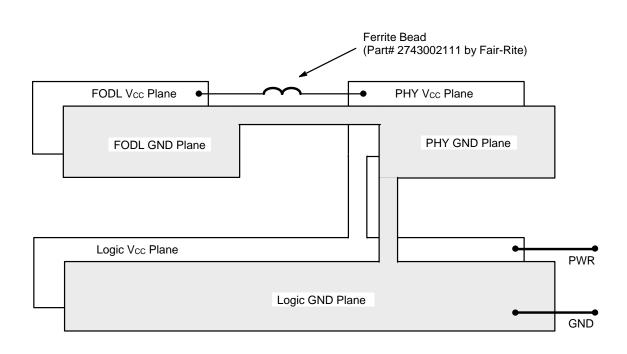
Figure 4. Fiber Optic Data Link Decoupling
