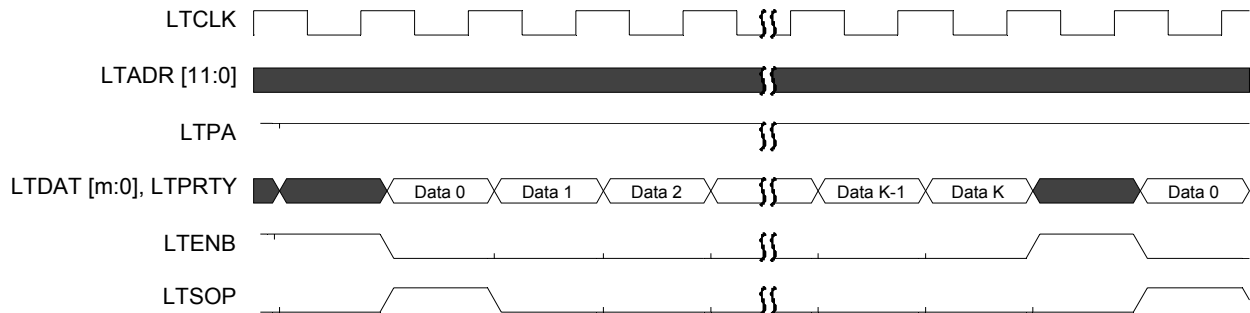
Figure 48 - Loop UTOPIA L1 Transmit Master
