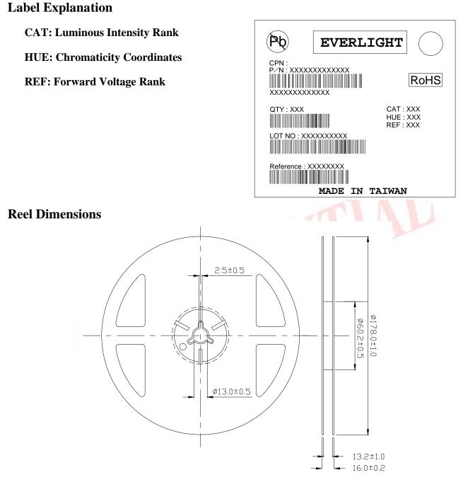
Note: The tolerances unless mentioned is ±0.1mm,Unit = mm
