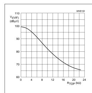
Typical tuner takeover point as a function of Fig.8 resistor R<sub>TOP</sub>.
