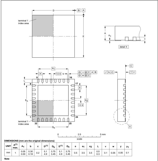
1. Plastic or metal protrusions of 0.075 mm maximum per side are not included.
