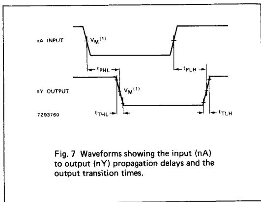
Fig. 7 Waveforms showing the input (nA) to output (nY) propagation delays and the output transition times.
