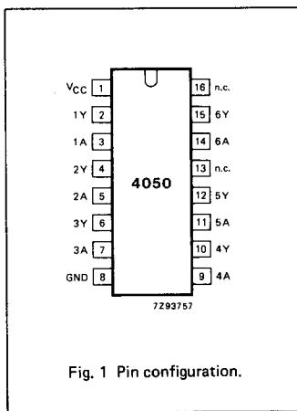
Fig. 1 Pin configuration.
