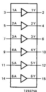
Fig. 4 Functional diagram.
