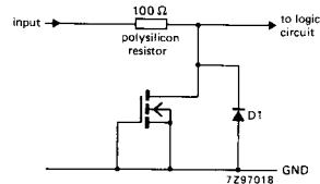
Fig. 5 Input protection for HC4050.
