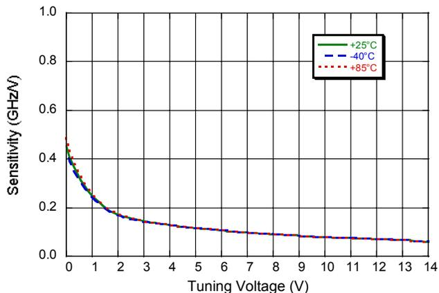
**Frequency Sensitivity vs. Tuning Voltage - RF/2 Port**
