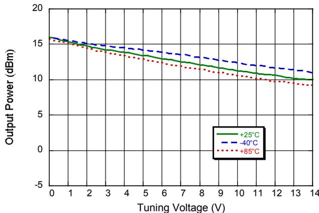
Output Power vs. Tuning Voltage - RF/2 Port
