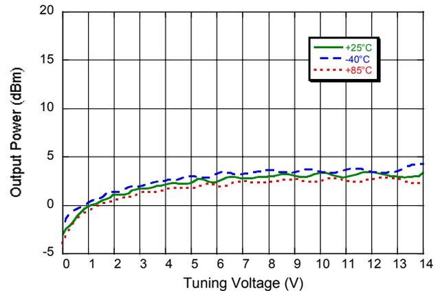
**Typical Performance Curves:  $V_{CC} = V_{BUFFER} = 5V$ ,  $T_A = +25^\circ C$  (unless otherwise indicated)**
