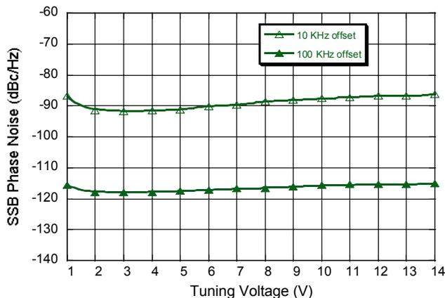
**Single Side Band Phase Noise vs. Frequency Offset
