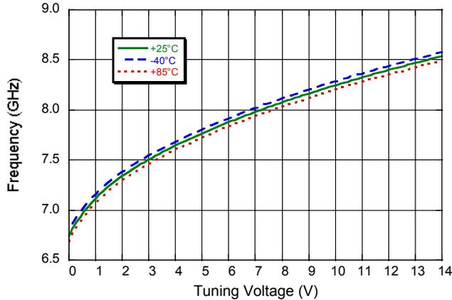
Output Frequency vs. Tuning Voltage - RF/2 Port
