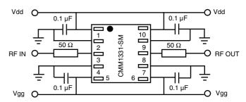
Note: Due to the high gain of this device it is highly recommended to maintain the reverse isolation (S12) above  $50 \, \mathrm{dB}$ .
