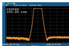
New 10-pole Collins® Mechanical SSB Filter Passband Response
