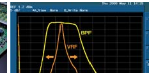
VRF Typical Bandpass Response (3.5 MHz)
