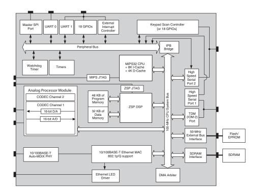
Broadcom's BCM1115 is designed for use in cost-sensitive, single Ethernet port consumer and Enterprise IP Phone and Gateway products.
