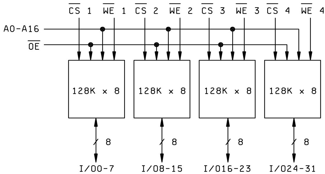
FIGURE 6. Block diagram(s).
