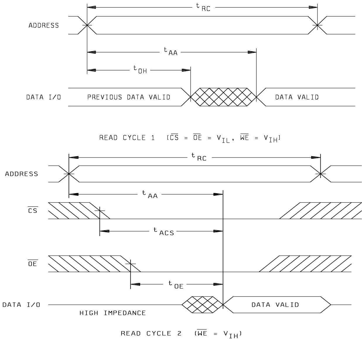
FIGURE 4. Read cycle timing diagram.
