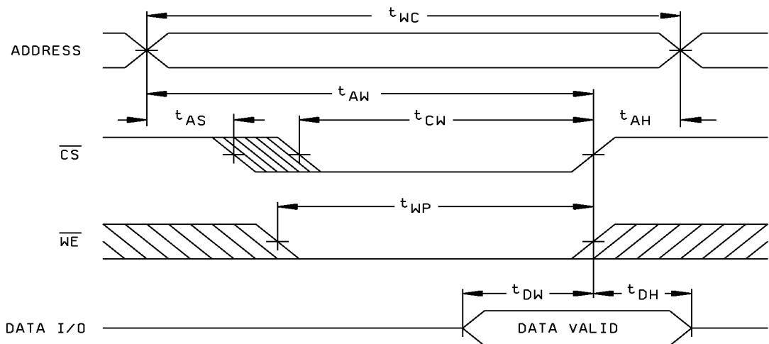
WRITE CYCLE 2  $\overline{CS}$  CONTROLLED
