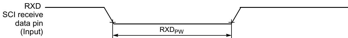
Figure 10-15 RXD Pulse Width
