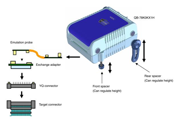
Figure 2-14. Connection Using Emulation Probe
