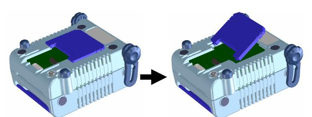
Figure 2-3. Acrylic Board Removal Method
