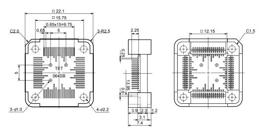
Figure B-30. Mount Adapter for 78K0/KE1 and 78K0/KE1+ (QB-64GC-HQ-01T)
