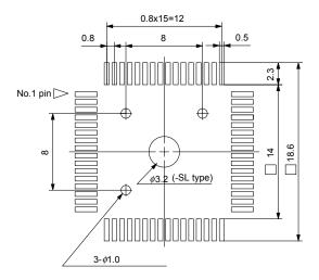
Figure B-7. Target Connector for 78K0/KF1 and 78K0/KF1+ (QB-80GK-NQ-01T)
