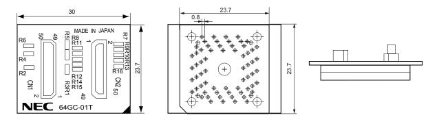
Figure B-15. Exchange Adapter for 78K0/KE1 and 78K0/KE1+ (QB-80GK-EA-01T)
