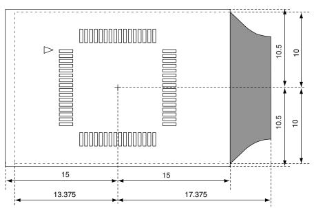
Figure A-5. For 78K0/KE1 or 78K0/KE1+ (64-Pin GK Package)
