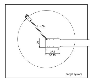
Figure 2-13. Where GND Wire Can Be Connected
