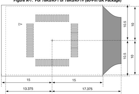
Figure A-7. For 78K0/KF1 or 78K0/KF1+ (80-Pin GK Package)
