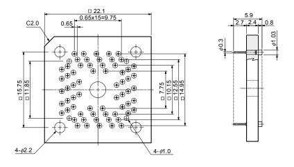
Figure B-39. Spacer Adapter for 78K0/KE1 and 78K0/KE1+ (QB-64GC-YS-01T)
