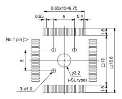
Figure B-6. Target Connector for 78K0/KE1 and 78K0/KE1+ (QB-64GC-NQ-01T) (1/2)
