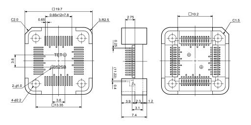
Figure B-28. Mount Adapter for 78K0/KE1 and 78K0/KE1+ (QB-64GB-HQ-01T)
