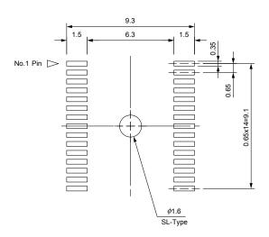
Figure B-2. Target Connector for 78K0/KC1 and 78K0/KC1+ (QB-44GB-NQ-01T)
