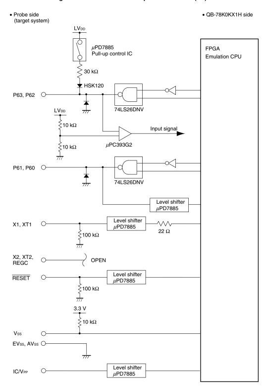
Figure 4-3. Emulation Circuit Equivalent Circuit 3 (2/2)
