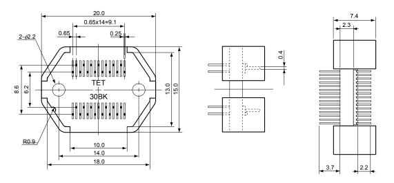
Figure B-18. YQ Connector for 78K0/KC1 and 78K0/KC1+ (QB-44GB-YQ-01T)
