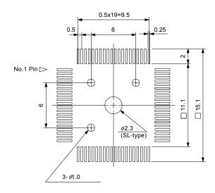
Figure B-8. Target Connector for 78K0/KF1 and 78K0/KF1+ (QB-80GC-NQ-01T)
