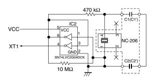
Remark Places surrounded by broken lines indicate portions installed on the parts board.
