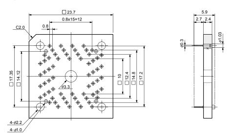
Figure B-40. Spacer Adapter for 78K0/KF1 and 78K0/KF1+ (QB-80GK-YS-01T)
