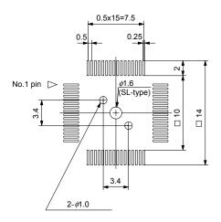
Figure B-5. Target Connector for 78K0/KE1 and 78K0/KE1+ (QB-64GK-NQ-01T)
