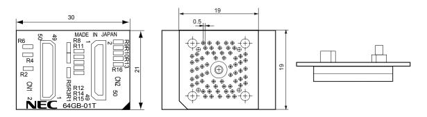
Figure B-13. Exchange Adapter for 78K0/KE1 and 78K0/KE1+ (QB-64GK-EA-01T)
