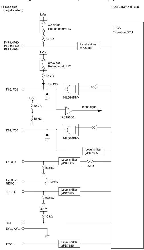
Figure 4-5. Emulation Circuit Equivalent Circuit 5 (2/2)
