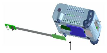
Insert CN1 and CN2 of the probe into TCN1 and TCN2 of the QB-78K0KX1H.
