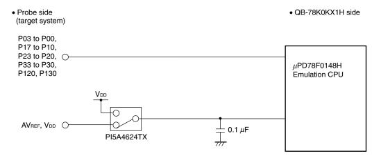
Figure 4-1. Emulation Circuit Equivalent Circuit 1 (2/2)
