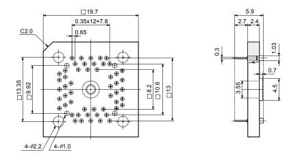
Figure B-37. Spacer Adapter for 78K0/KE1 and 78K0/KE1+ (QB-64GB-YS-01T)
