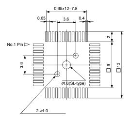
Figure B-4. Target Connector for 78K0/KE1 and 78K0/KE1+ (QB-64GB-NQ-01T)
