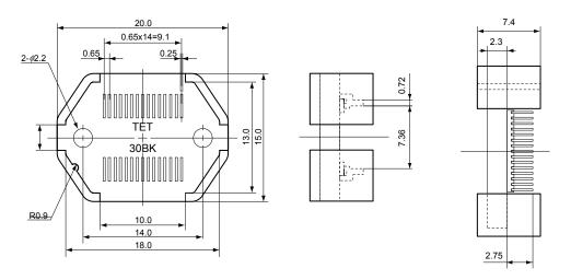
Figure B-26. Mount Adapter for 78K0/KC1 and 78K0/KC1+ (QB-44GB-HQ-01T)
