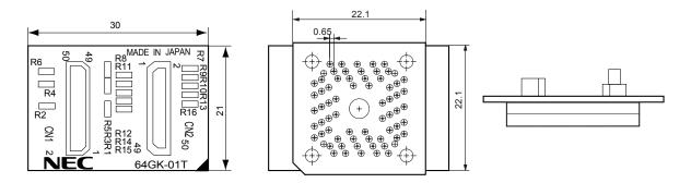
Figure B-14. Exchange Adapter for 78K0/KE1 and 78K0/KE1+ (QB-64GC-EA-01T)
