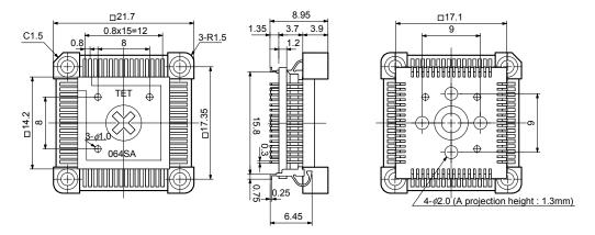
Figure B-6. Target Connector for 78K0/KE1 and 78K0/KE1+ (QB-64GC-NQ-01T) (2/2)
