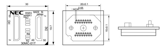
Figure B-10. Exchange Adapter for 78K0/KC1 and 78K0/KC1+ (QB-44GB-EA-01T)
