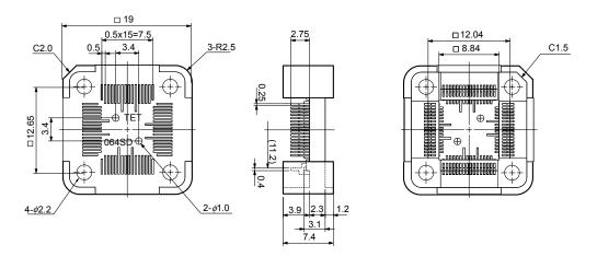
Figure B-29. Mount Adapter for 78K0/KE1 and 78K0/KE1+
