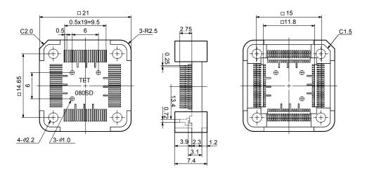
Figure B-32. Mount Adapter for 78K0/KF1 and 78K0/KF1+ (QB-80GC-HQ-01T)
