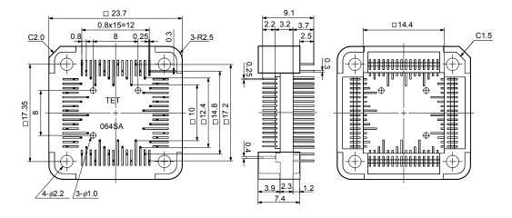
Figure B-23. YQ Connector for 78K0/KF1 and 78K0/KF1+ (QB-80GK-YQ-01T)
