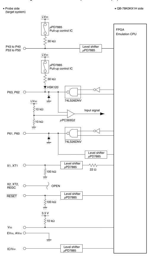
Figure 4-4. Emulation Circuit Equivalent Circuit 4 (2/2)
