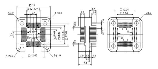
Figure B-21. YQ Connector for 78K0/KE1 and 78K0/KE1+ (QB-64GK-YQ-01T)
