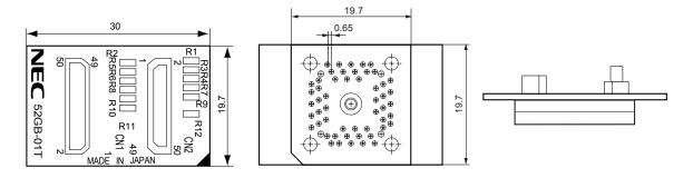
Figure B-12. Exchange Adapter for 78K0/KE1 and 78K0/KE1+ (QB-64GB-EA-01T)
