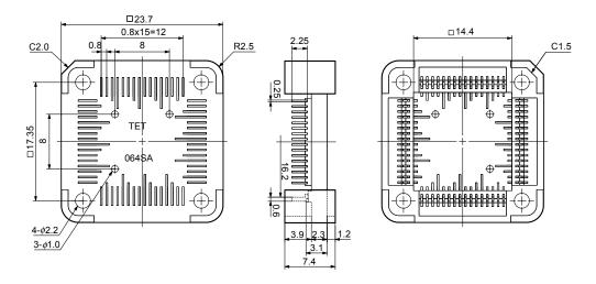
Figure B-31. Mount Adapter for 78K0/KF1 and 78K0/KF1+ (QB-80GK-HQ-01T)
