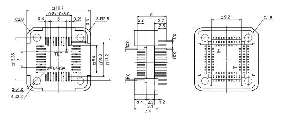
Figure B-19. YQ Connector for 78K0/KD1 and 78K0/KD1+ (QB-52GB-YQ-01T)
