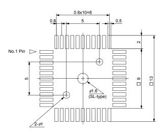
Figure B-3. Target Connector for 78K0/KD1 and 78K0/KD1+ (QB-52GB-NQ-01T) (1/2)
