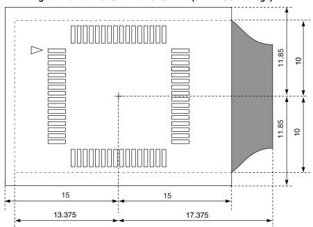
Figure A-6. For 78K0/KE1 or 78K0/KE1+ (64-Pin GC Package)
