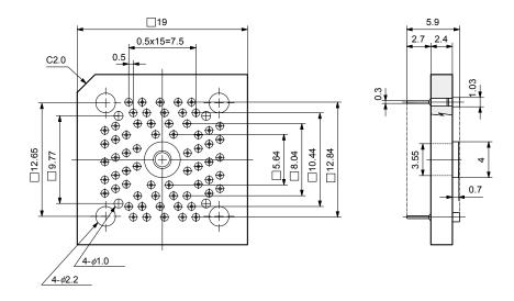
Figure B-38. Spacer Adapter for 78K0/KE1 and 78K0/KE1+ (QB-64GK-YS-01T)
