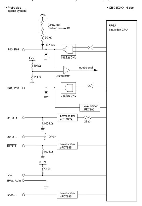
Figure 4-2. Emulation Circuit Equivalent Circuit 2 (2/2)
