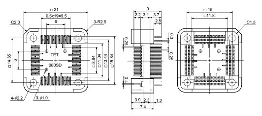
Figure B-24. YQ Connector for 78K0/KF1 and 78K0/KF1+ (QB-80GC-YQ-01T)
