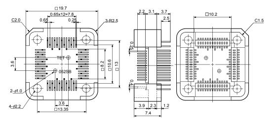
Figure B-20. YQ Connector for 78K0/KE1 and 78K0/KE1+ (QB-64GB-YQ-01T)
