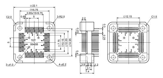
Figure B-22. YQ Connector for 78K0/KE1 and 78K0/KE1+ (QB-64GC-YQ-01T)
