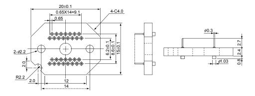
Figure B-35. Spacer Adapter for 78K0/KC1 and 78K0/KC1+ (QB-44GB-YS-01T)
