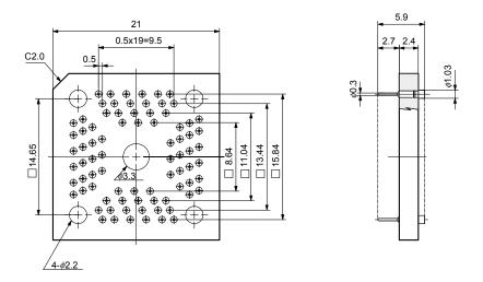
Figure B-41. Spacer Adapter for 78K0/KF1 and 78K0/KF1+ (QB-80GC-YS-01T)
