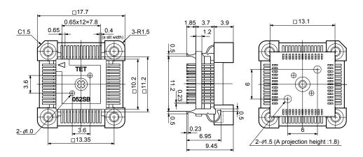
Figure B-3. Target Connector for 78K0/KD1 and 78K0/KD1+ (QB-52GB-NQ-01T) (2/2)
