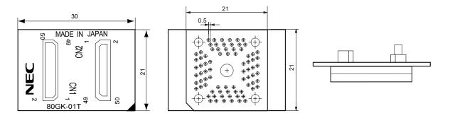
Figure B-16. Exchange Adapter for 78K0/KE1 and 78K0/KE1+ (QB-80GC-EA-01T)
