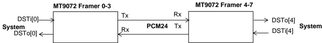
e) *Framer ST-BUS loopback(Register 904)* - Internally connects DSTi of one framer to DSTo of one of the other integrated framers.
