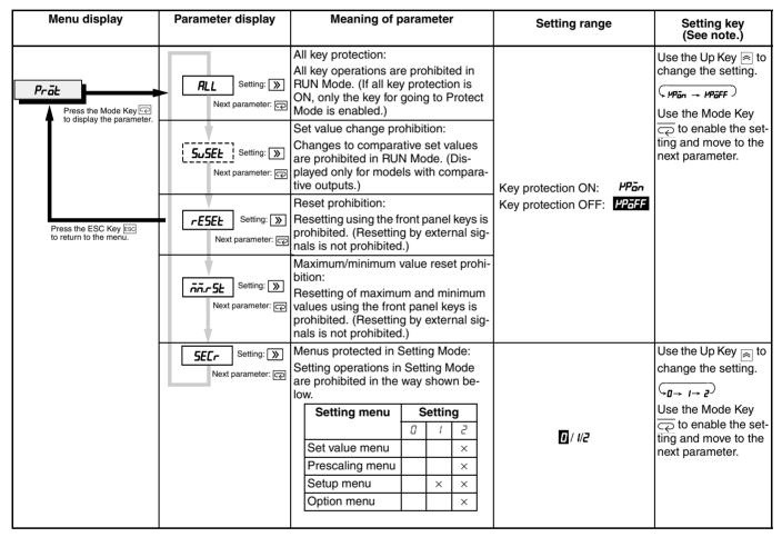
Note: If there is no key operation for 5 seconds, the setting is automatically registered.
