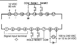
Transistor Inputs: ON: Residual voltage must be 3 V max.
