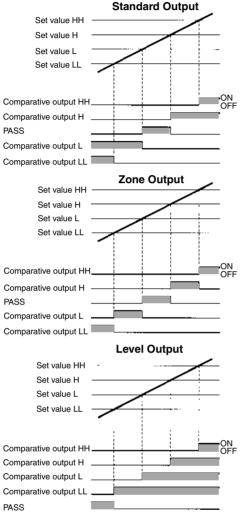
Note: The following setting conditions must be satisfied, otherwise no zone output will turn ON correctly.
