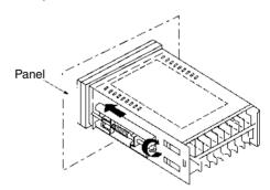
Attach the mounting bracket on the left and right sides of the Frequency/Rate Meter as shown in the illustration above and gradually tighten each screw evenly in turn by considering the balance of the tightening force until the ratchets start slipping without being further
