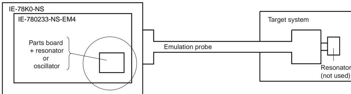
**Remark** The clock that is supplied by the IE-780233-NS-EM4's resonator or oscillator (encircled in the figure) is used.
