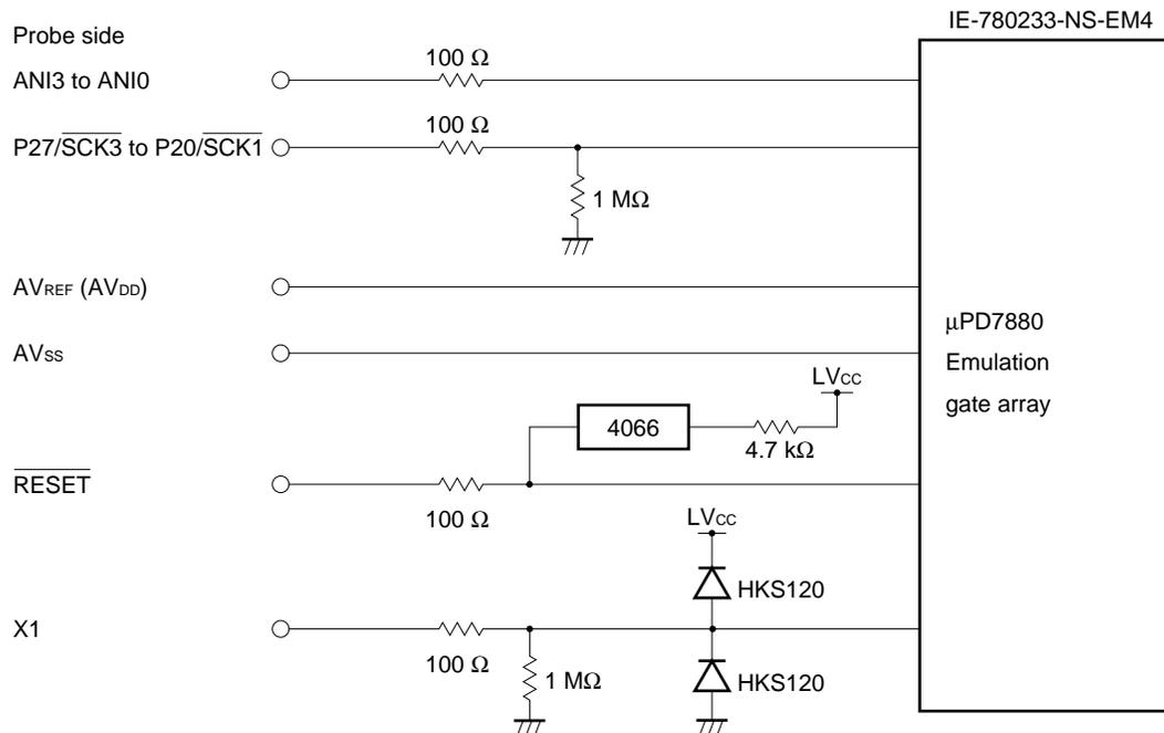
Figure 4-2. Equivalent Circuit of Emulation Circuit 2
