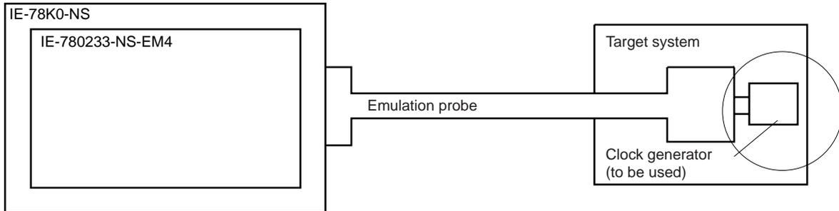
**Remark** The clock supplied by the target system's clock generator (encircled in the figure) is used.
