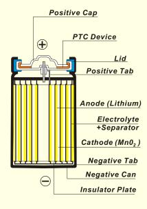
Fig.3 Spiral construction Schematic construction of a Li/MnO<sub>2</sub>cylindrical cell (CR 123A)
