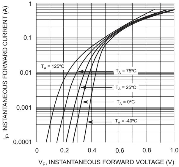
Fig. 1 Forward Characteristics
