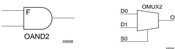
Figure 20: AND & MUX Symbols in XC4000X IOB
