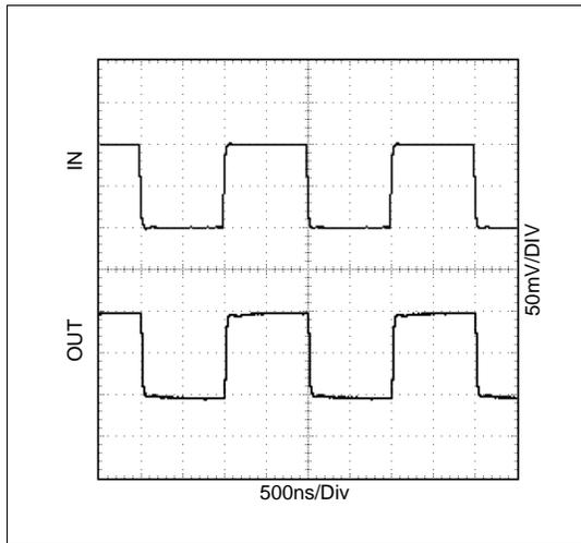
Figure 16. Transient Response, 100mV, 100pF load
