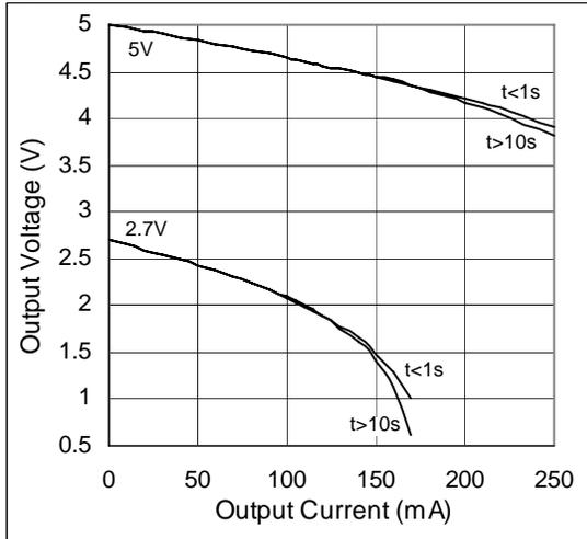
Figure 12. Output Voltage vs. Output Current, sinking
