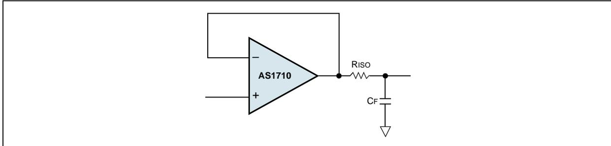
**Note:** Resistor RISO improves the circuit's phase margin by isolating the load capacitor from the AS1710/AS1712 output.
