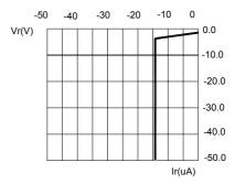
FIG.2 REVERSE CURRENT VS. REVERSE VOLTAGE.
