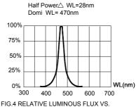
FIG.4 RELATIVE LUMINOUS FLUX VS. WAVELENGTH.
