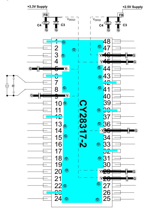
**③** = VIA to GND plane layer **○** ■ VIA to respective supply plane layer
