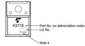
Note 4: A line under a Lot No. identifies the indication of product Labels. Not underlined: [[Pb]]/INCLUDES > MCV Underlined: [[G]]/RoHS COMPATIBLE or [[G]]/RoHS [[Pb]]
