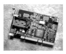
connection. An HSSDC connector is available for intra-cabinet connectivity, while a GBIC (copper or optical) provides external connectivity. System vendors can utilize either one or both of the connectors simultaneously.
